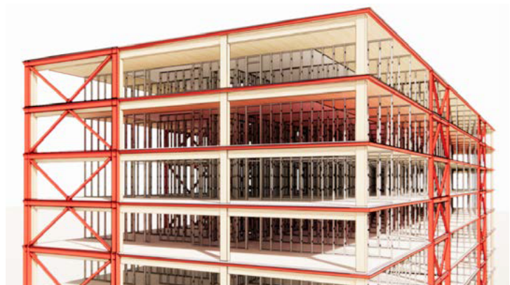
Figure 7. CLT/CFS with lateral load resisting system (LLRS) steel braced frame (image courtesy Timber Engineering, Inc)
