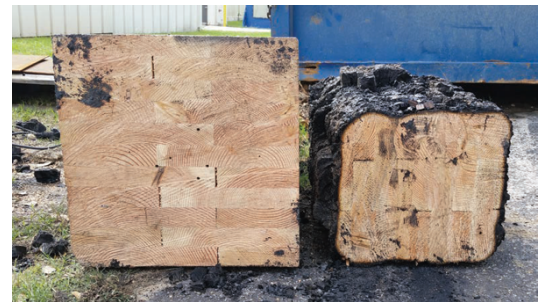
Figure 3. Glulam column before and after 2-hour fire test. Photo: David Barber, Arup
